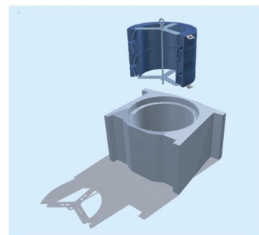
Fig7-9 : Mounting a sealed four-row tapered roller bearings
