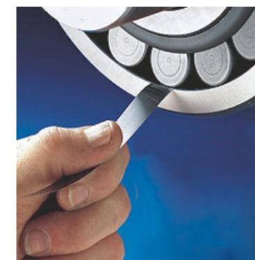
Fig. 4-4 : Bearing clearance measurement
